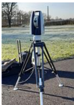
Photo 4: Reference positioning tool (XYZ precision 1/100 mm)
