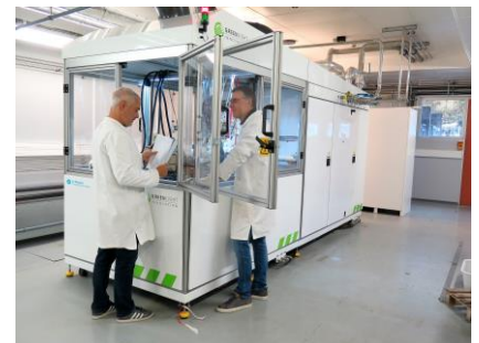
Photo 3: Test bench for 100 kW fuel cells - CEA
